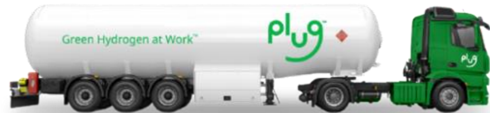
LH2 Tanker Capacity = 4900 kg
