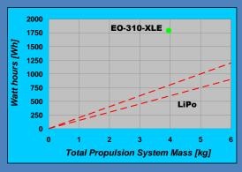
The output voltage range of the EO-310-XLE is similar to that of an 8 to 10S LiPo battery pack, which eliminates the need for any power conditioning between the fuel cell system and your propulsion motor (i.e. a heavy and inefficient DC/DC converter is not required).
