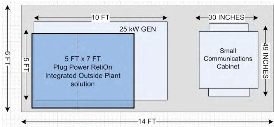
Up to 58% footprint savings using Plug Power's GenSure Integrated Outside Plant solution compared to a small communications cabinet and combustion generator. Versus a small communications shelter and the same combustion generator, 87% footprint savings.
