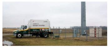
the fuel to supply electricity and there are options for fueling. Traditionally, fuel cells have used hydrogen cylinders to store fuel (packaged gas). The refueling of hydrogen cylinders is accomplished by a vehicle transporting full cylinders to the site and exchanging them for the empty cylinders. Though labor-intensive, this remains the option of choice for many locations.
