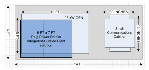
Up to 58% footprint savings using Plug Power's ReliOn Integrated Outside Plant solution compared to a small communications cabinet and combustion generator. Versus a small communiations shelter and the same combustion generator, 87% footprint savings.
