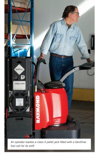
Operators also like the system because GenDrive provides full power throughout the shift, while lead-acid batteries degrade, affecting operator efficiency and potentially impacting their job and incentives.
